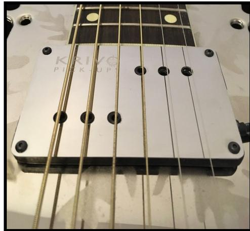
4. Gently, but firmly, press the pickup down using a slight rocking motion until it is securely affixed to the guitar.
